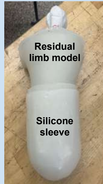
Figure 4: Silicone Sleeve Integration with Residual Limb Model.
